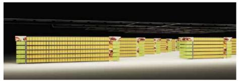
Although products are sufficiently illuminated, homogeneous grid lighting does not provide highlights or points of interest.
