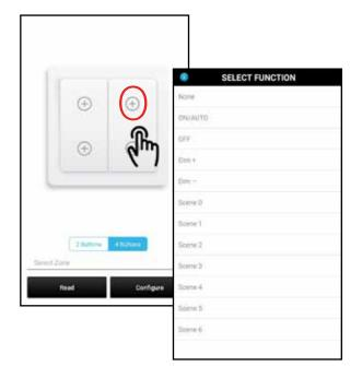
NOTE: Each EnOcean push button panel can control one zone. If no zone is selected the push button will control all zones within Radio Range.
